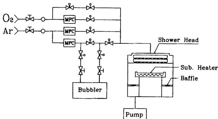
FIGURE 1 Schematic diagram of MOCVD apparatus.
