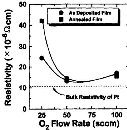
FIGURE 7 Electrical resistivities of Pt thin films deposited with the addition of various amount of O<sub>2</sub> during the deposition.
