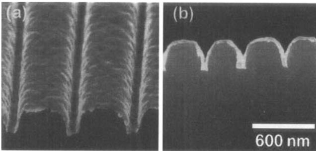
FIGURE 8 SEM micrograph of Pt thin films deposited on patterned SiO<sub>2</sub>/Si at 350°C : (a) top view and (b) cross-sectional view.
