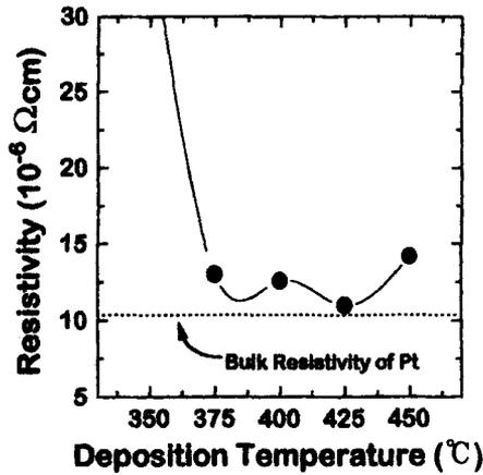
FIGURE 4 Electrical resistivities of Pt thin films deposited at various substrate temperatures.
