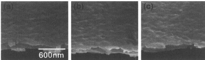
FIGURE 6 SEM micrographs of Pt thin films deposited on BST/Pt/SiO<sub>2</sub>/Si at 350°C with the addition of  $O_2$  gas of (a) 25 sccm, (b) 50 sccm and (c) 100 sccm.
